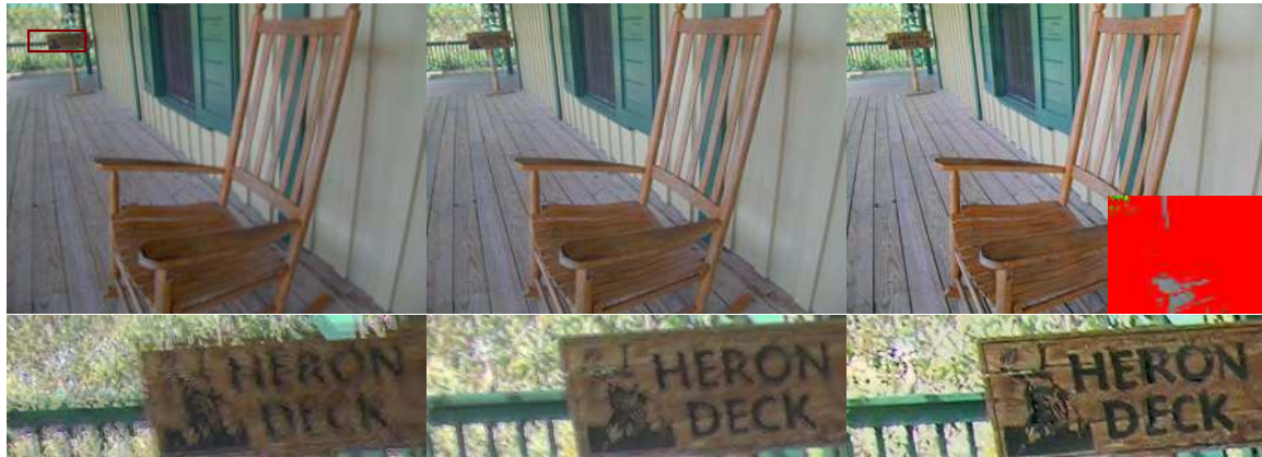
Figure 4: Left: Unaligned HDR image created from hand-held exposures. Middle: Exposures aligned using the MTB algorithm. Right: Our result. The close-ups demonstrate that our algorithm produces sharper images. The color map shows the source exposures for different regions of the HDR image.
