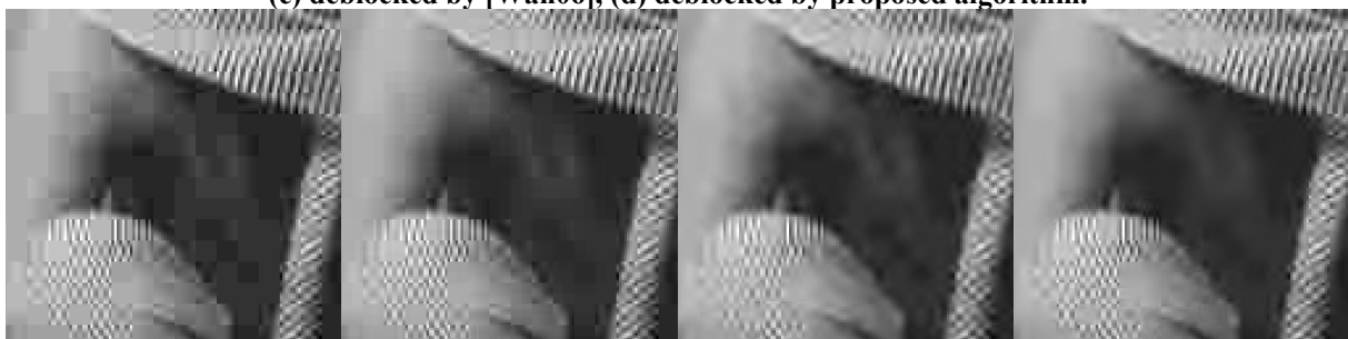
(a) (b) (c) (d) Figure 8. Enlarged Barbara : (a) JPEG decoded (0.306bpp), (b) deblocked by [Luo03], (c) deblocked by [Wan06], (d) deblocked by proposed algorithm.
