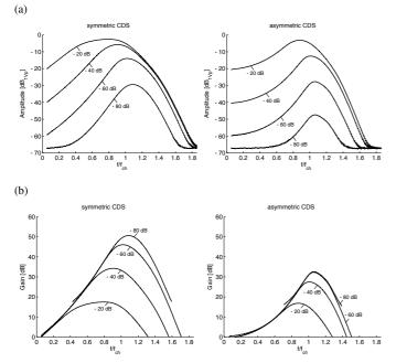
Fig. 1. Single tone responses, section 8,  $f_{ch} = 2960 \text{ Hz}$  and  $\mu_i = -0.2 \forall i$ .
