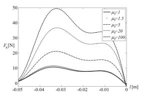
FIG.2.: STATIC CHARACTERISTICS OF THE HORIZONTAL FORCE OF ELECTROMECHANICAL ACTUATOR FOR FERROFLUIDS WITH DIFFERENT PERMEABILITIES
