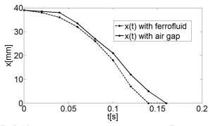
FIG.3.: MEASURED DYNAMIC CHARACTERISTICS OF THE EXPERIMENTAL LINEAR ELECTROMECHANICAL ACTUATOR
