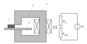
Fig.1.: Simple electromechanical actuator and its equivalent magnetic circuit; 1 - movable part, 2 -magnetic circuit, 3 - winding, 4 - air gap between movable and static part
