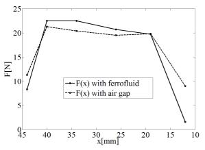
FIG.4.: MEASURED STATIC CHARACTERISTICS OF THE EXPERIMENTAL LINEAR ELECTROMECHANICAL ACTUATOR
