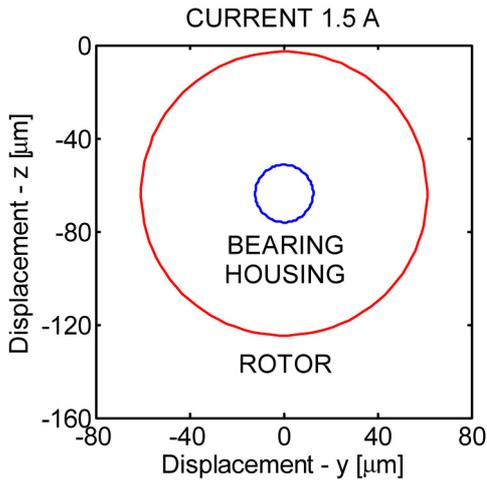
Fig. 7. Rotor and bearing housing centre orbits
