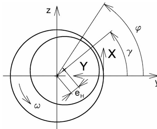
Fig. 3. Coordinate systems of the damper
