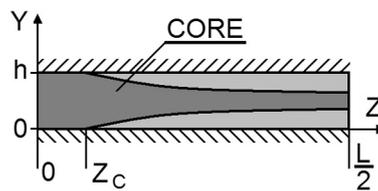
Fig. 4. The core formation in the lubricating film
