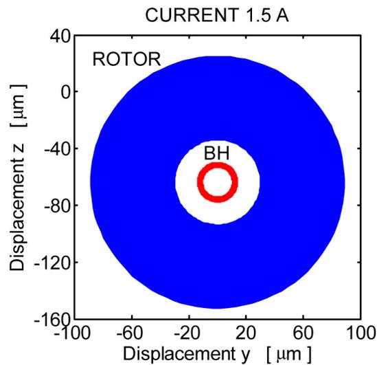
Fig. 11. Rotor orbit (BH-bearing housing)
