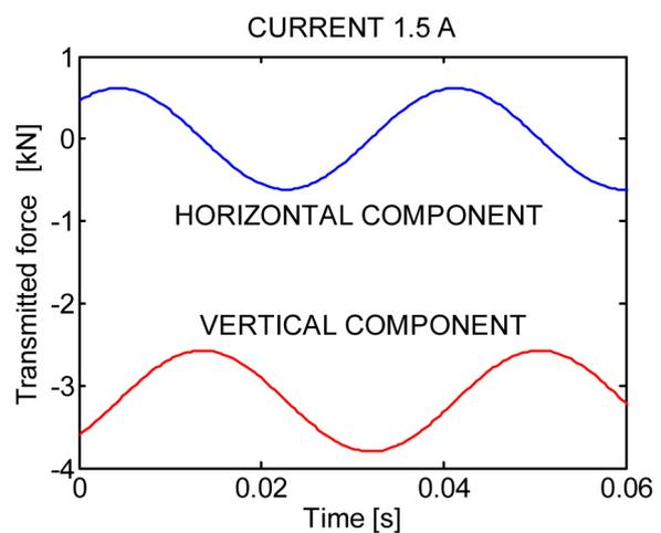
Fig. 8. Transmitted force components (nominal speed)
