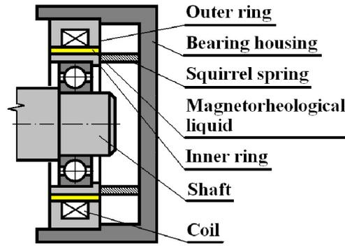
Fig. 2. Magnetorheological damper
