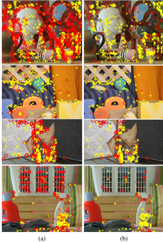
Figure 2: The two image-based matching approach (a) results in more outliers (red circles) and a lower relative amount of inliers (yellow crosses) than our three image based-matching (b). From top to bottom: scene art with SIFT features, RubberWhale with SURF features, stonemill with Harris corners, laundry with FAST features, all using nearest neighbor matching.
