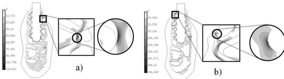
Fig. 13. 1st Principal stress. Stage C: a)  $T(0.47) - 0.1$ , b)  $T(0.32) - 0.1$
