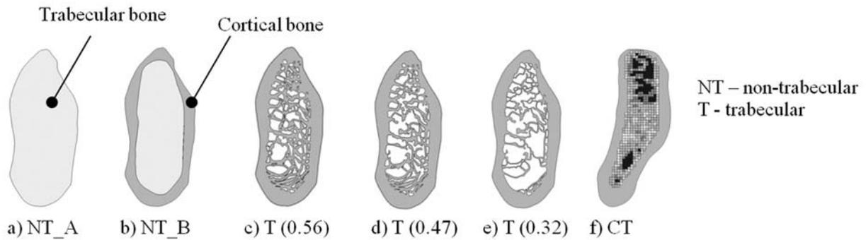
Fig. 1. Model of geometry and analyzed material modeling levels overview: a) non-trabecular model (only cancellous bone) – NT\_A; b) non-trabecular model (cancellous as well as cortical bone) – NT\_B; c) trabecular bone of good quality (BA/TA – 0.56); d) trabecular bone of normal quality (BA/TA – 0.47); e) trabecular bone of low quality (BA/TA – 0.32); f) CT-obtained model
