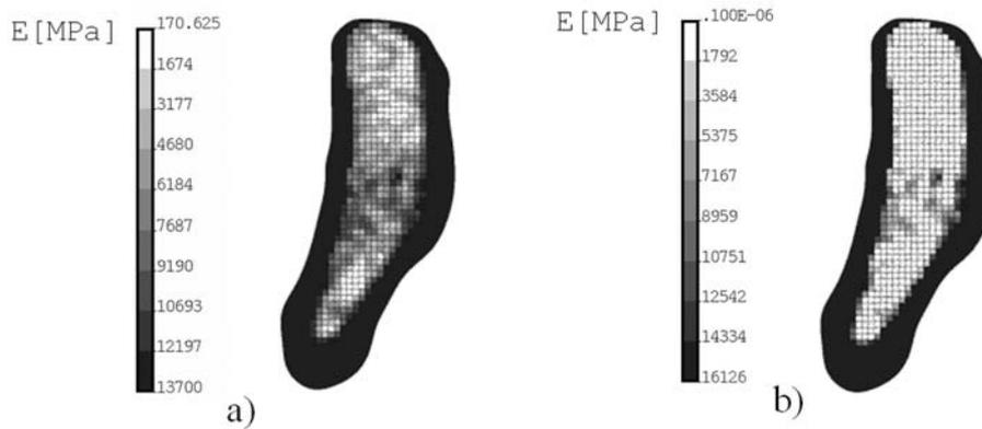
Fig. 2. CT-obtained material model: a) linear correlation used – CTlin, b) nonlinear correlation used – CTnonlin
