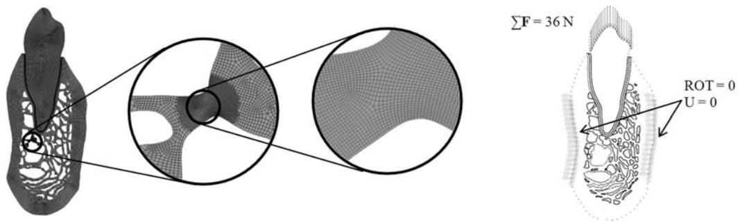
Fig. 4. FE mesh and the boundary condition
