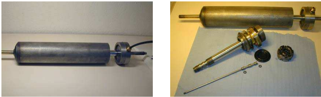
Fig. 1. The air-pressure-controlled hydraulic shock absorber and its structural members
