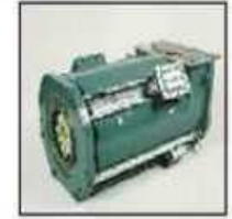
Double motor for Sprint Tram Amsterdam. Self ventilated motor 2 x 74 kW.
