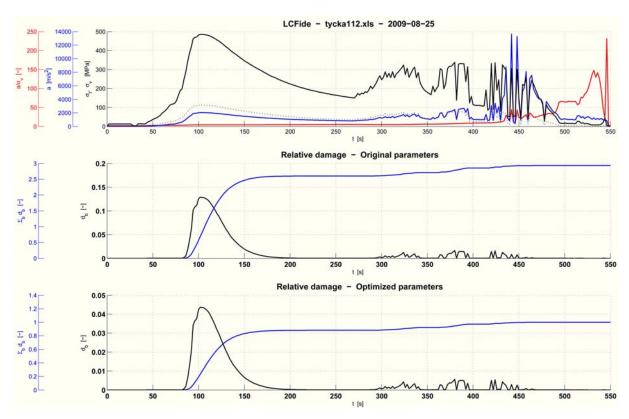
Fig. 1. Vibrational data (a), estimated damage (b), optimized damage (c)
