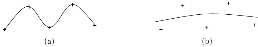
Figure 2: Two possibilities of fitting the function to the set of points: (a) interpolation, (b) approximation
