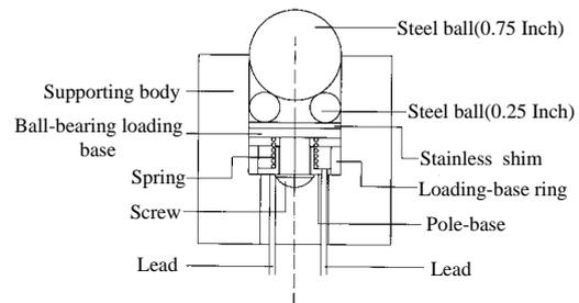
Figure 3. A cross-sectional view of the position sensor
