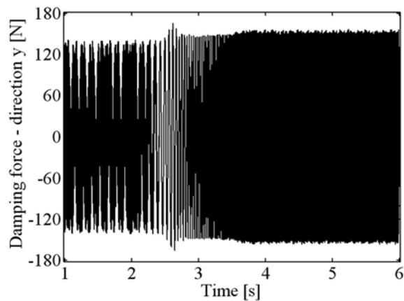
Fig. 16. Force transmitted to the foundations (2 A)
