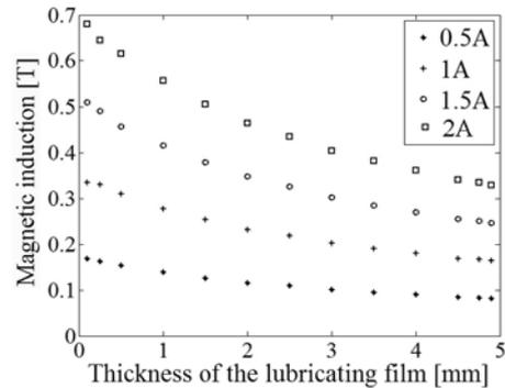
Fig. 8. The flux density – thickness relationship
