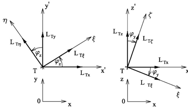
Fig. 3. Coordinate systems and components of the rotor moment of momentum  $L_{Tx}$ ,  $L_{Ty}$ ,  $L_{Tz}$ ,  $L_{T\xi}$ ,  $L_{T\eta}$ ,  $L_{T\zeta}$  denote components of the moment of momentum of the rotor
