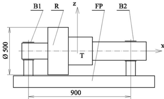
Fig. 10. Scheme of the rotor
