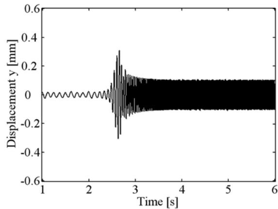
Fig. 14. Horizontal displacement of the rotor (2 A)
