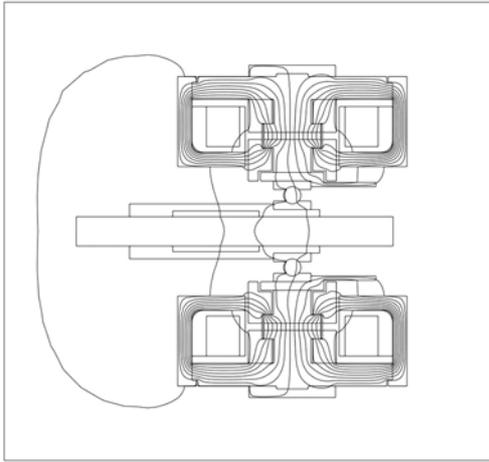
Fig. 5. The magnetic field distribution, (2.5–2.5) mm, 1 A
