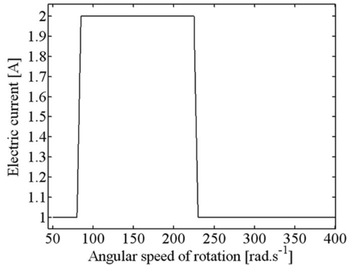
Fig. 17. The current – speed of rotation relationship
