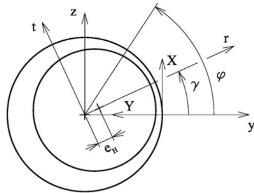
Fig. 2. The damper coordinate system
