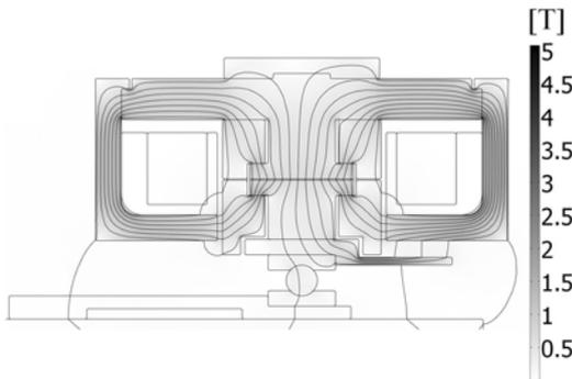
Fig. 7. The magnetic field, 0.25 mm, 2 A
