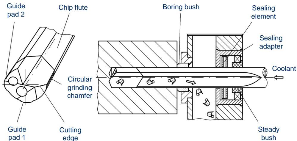
Figure 1: Schematic illustration of the single-lip deep hole drilling [5]
