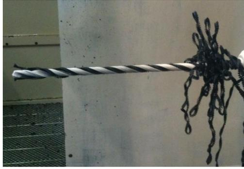
Figure 5: *Looped chips at the tool shank*
