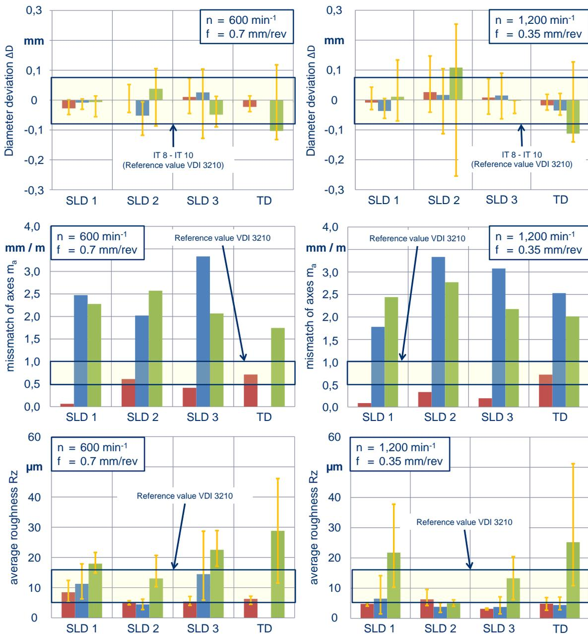
Figure 3: Results of the deep hole drilling of POM, PA and PE
