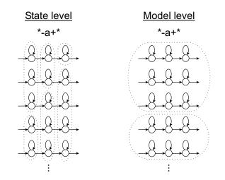
Fig. 2. An illustration of state-level (left) and model-level clustering (right) of all triphones derived from the phoneme /a/. Dotted lines show the examples of the resulting clusters.
