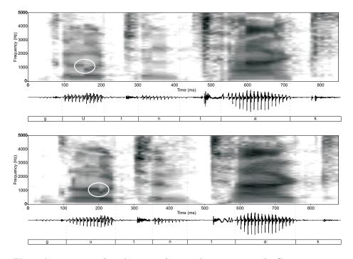
**Fig. 3.** A comparison of synthetic waveforms and spectrograms of a German sentence "*Guten Tag.*" when using fenemes (top) or triphones (bottom) as speech units. White oval shows an example of a within-phoneme formant discontinuity typical for feneme-based synthesis. Dotted lines show phoneme boundaries in the synthetic speech.
