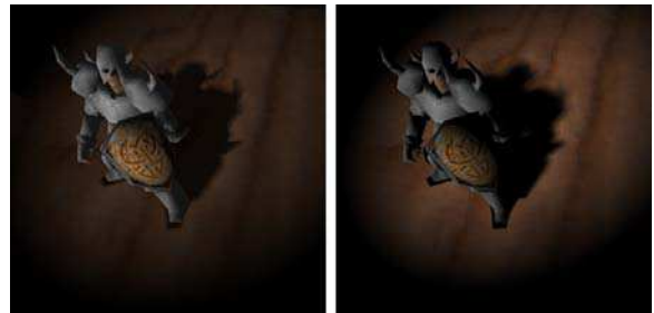
Figure 5. A test scene with non-trivial shadow casting objects (2148 triangles). The left image is generated with penumbra maps while the right image is generated with 128 supersampled shadow map images.
