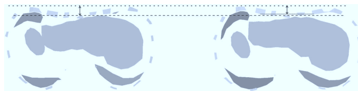
Fig. 9. Bottom torso deflection, when a) no airbag, b) airbag was used during the 50 km/h test
