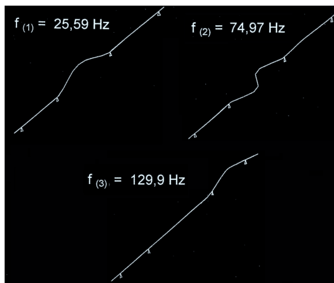
Fig. 5. The first three natural modes of rotor axis.
