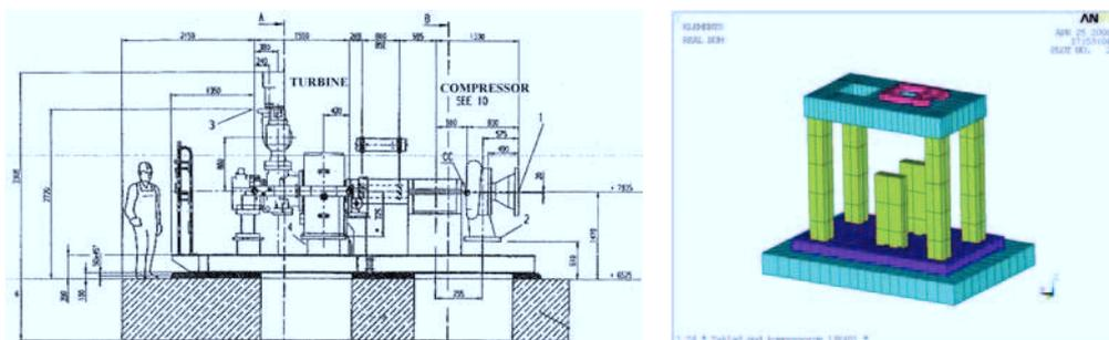
Fig. 4. Scheme of compressor 13K401 and foundation FEM model
