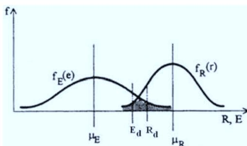
Fig. 1. Functions of the probability density  $f_R(r)$  and  $f_E(e)$
