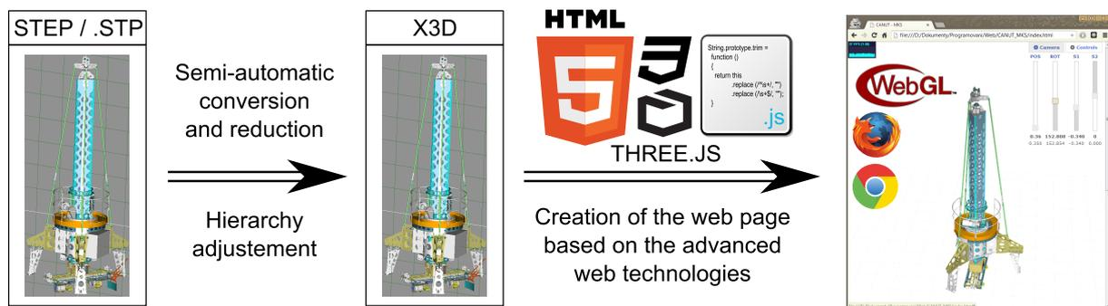
**Figure 1:** Process of creation of the visualization
