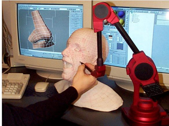
**Figure 5.2:** Digitizing a head using MicroScribe digitizer (from [1])
