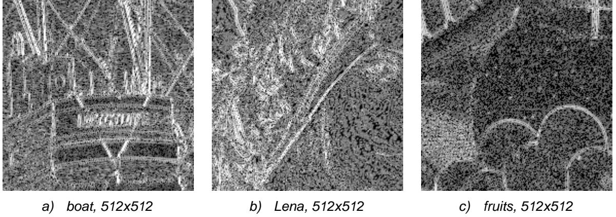
Figure 3.7: The significance map computed by the DISTW method for small areas of three popular grey-scale images. Lighter pixels represent more significant points.
