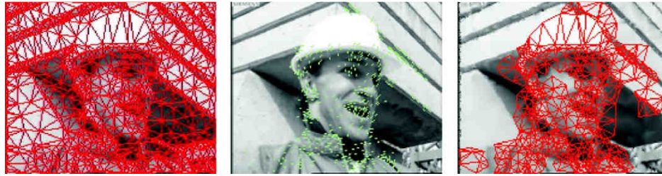
Figure 8.5: The original KDT, detected motion vectors and the movement compensation in the KDT.
