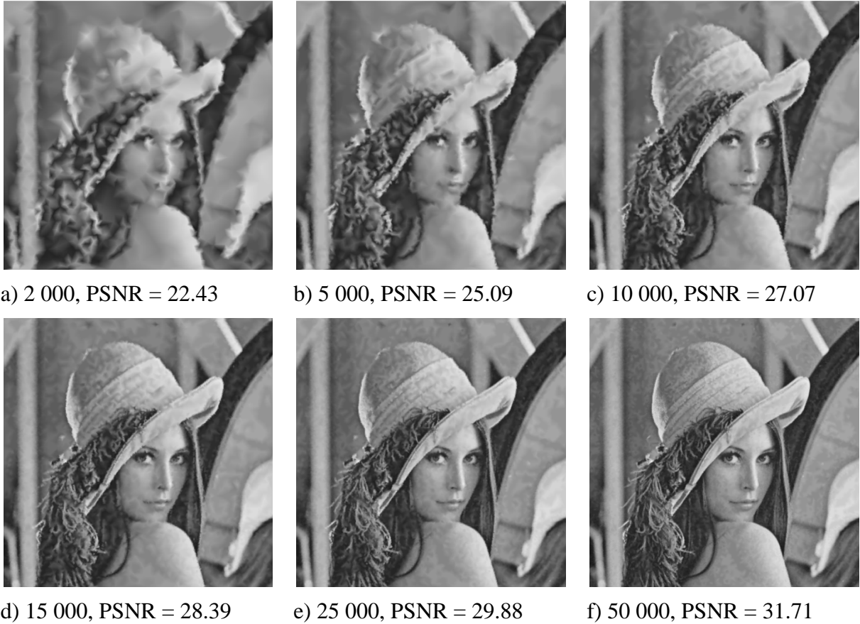
Figure 4.15: The comparison of Lena images reconstructed from triangulations with various vertices computed by the ERRDIST method combined with the GAUSS method with when the influence factor ( \sigma ) 8 and the vicinity area ( r ) 16.
