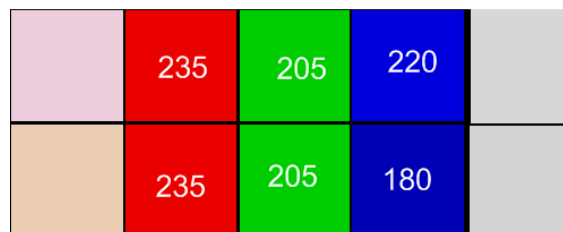
Figure 7.7: Illustration of colour bleeding – top: the original colour, its RGB components and the corresponding grey-scale value; bottom: the colour reconstructed with an error in the blue component.
