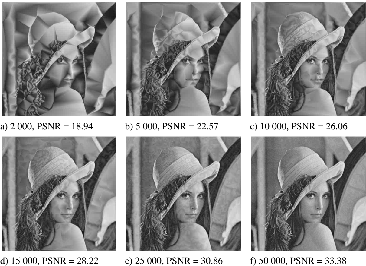
Figure 4.8: The comparison of Lena images reconstructed from triangulations with various vertices computed by the DISTW method.
