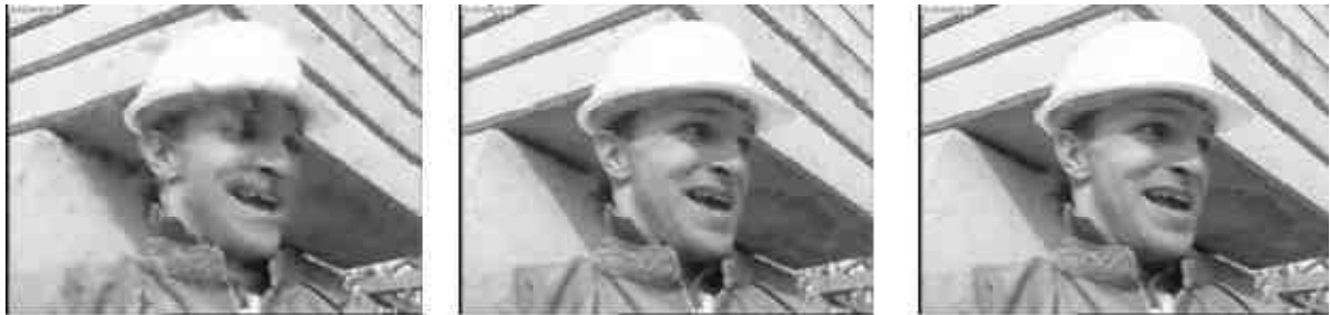
Figure 8.11: Comparison of the image reconstructed from the Delaunay triangulation of 20% points selected by proprietary refinement technique (left), the BRUTE decimation technique (middle) with the image that was subject to M-JPEG compression.
