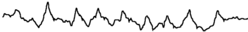
Fig. 48: The results of 8 pulses burning in distance 52 \mu\text{m} with the inaccuracy 10 \mu\text{m} into cermet in the top view and as the horizontal cross-section curve.
