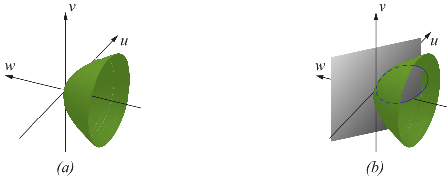
Figure 3.8: Paraboloid of revolution. (a) Components identical to objects waves and (b) intersection between the paraboloid of revolution and a sectional Fourier plane. [SIY04]
