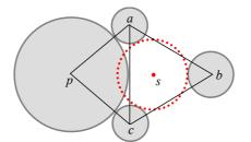
Fig. 5.4: The center of the circle s lies in the orthogonal center of a triangle abc. The circle s does not have any intersection with the atoms a, b, c, but it still intersects the atom p.
