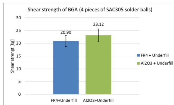
Fig. 7: Shear strength of BGA soldered on FR4 and alumina substrates with underfill
