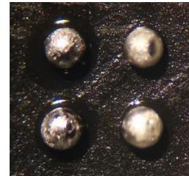
Fig. 4: Dummy BGA with solder balls
