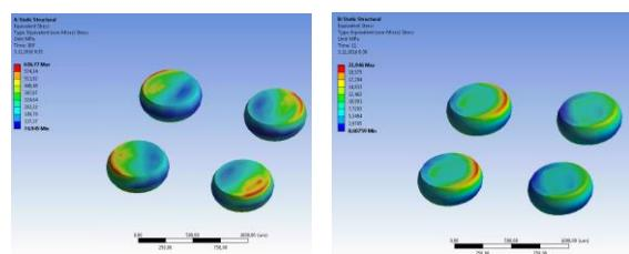
Fig. 8: Equivalent stress at solder balls without underfill (left) and with underfill (right)
