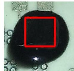
Fig. 5: Soldered BGA on alumina with underfill
