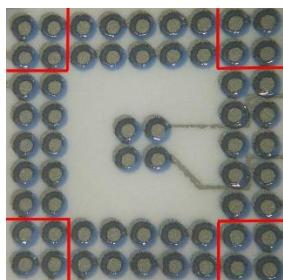
Fig. 3: Alumina substrate with marked positions of place for BGA assembly
