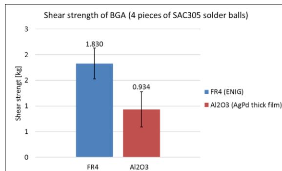
Fig. 6: Shear strength of BGA soldered on FR4 and alumina substrates
