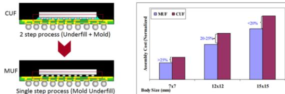
Fig. 2: Difference between CUF and MUF technology [5]
