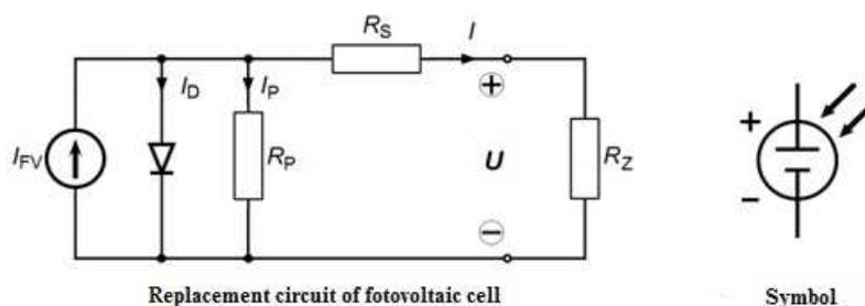
Figure 1 – Replacement circuit of photovoltaic cell
