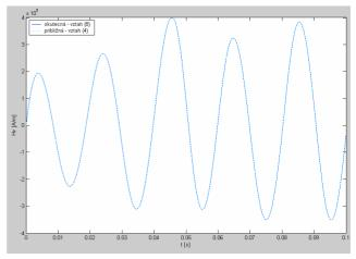
Fig. 4: Comparison of the behaviour of time dependences of  $H_V$  according to the formula (4) a (8)
