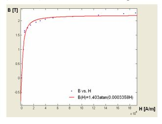
Fig. 2: Field characteristic of the magnetic circuit of the actuator
