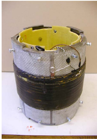
Fig. 9. Primary and secondary coil
