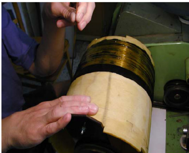
Fig. 11. Superconducting wire coiling
