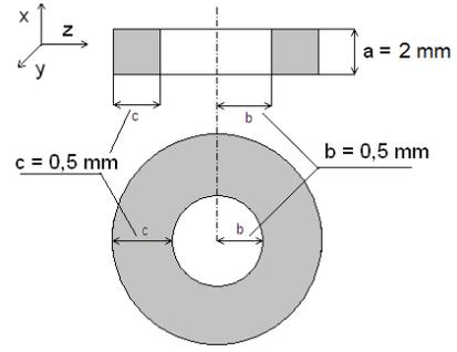
Fig.5: Dimension of the absolute coil
