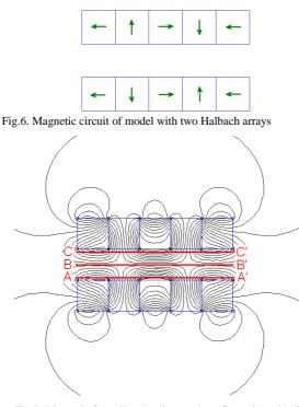
Fig.7. Magnetic force lines in discussed configuration with lines A-A', B-B'and C-C'
