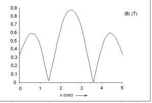
Fig.11. Magnetic flux density absolute value along line B-B'
