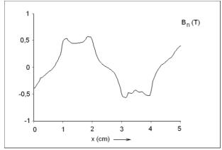
Fig.9. Magnetic flux density normal part value along line A-A
