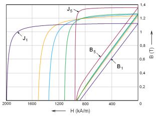
Fig.1. Sintered NdFeB permanent magnets demagnetization curves
