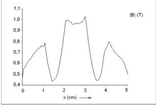
Fig.8. Magnetic flux density absolute value along line A-A' (and line C-C')
