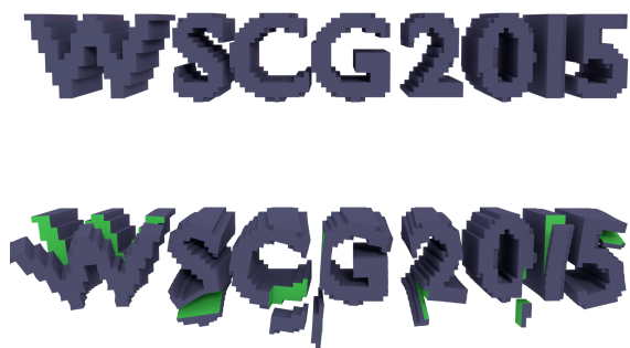
Figure 10: Cutting made during a MSS simulation. Some particles were fixed and the gravity was applied. The density of the letters was put to \rho = 200 \text{ Kg.m}^{-3} .
