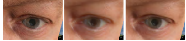
Figure 6: Reducing blur between skin and non-skin zones: without subsurface scattering (left), simple subsurface scattering (centre), and using a bilateral filter to avoid blurring between skin and non-skin zones (right).
