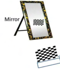
Figure 3: The Kinect camera can see the checkerboard through the mirror
