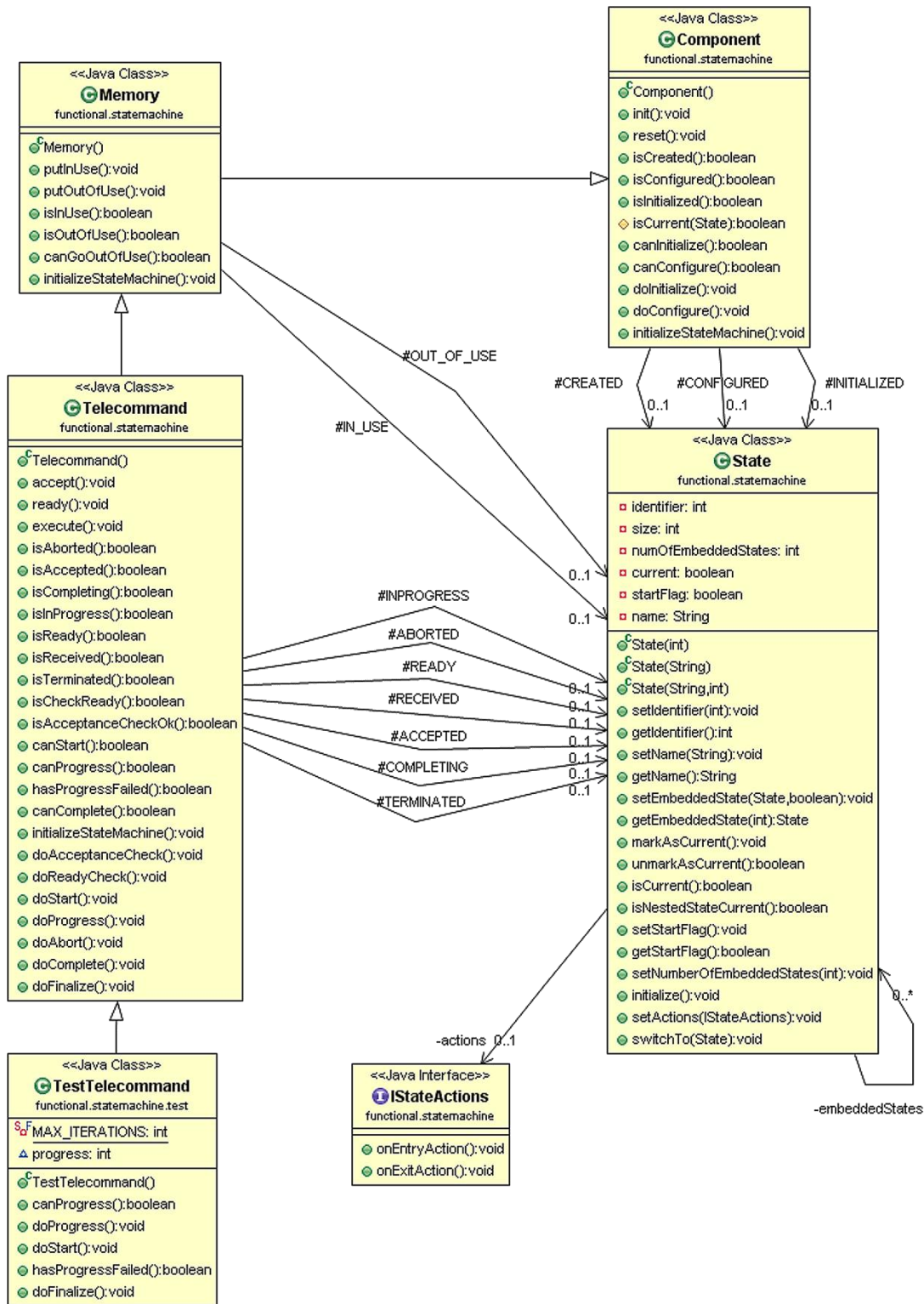
Figure 47 – Class diagram of Telecommand
