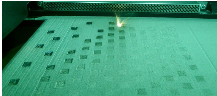
Fig. 7. Experimental samples (cubes) during the sintering process
