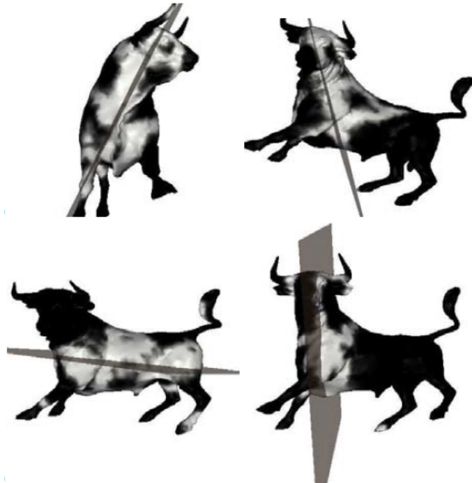
Figure 2.7: Several symmetry planes detected using the method by Podolak et al. on a single object. (Figure taken from [17].)
