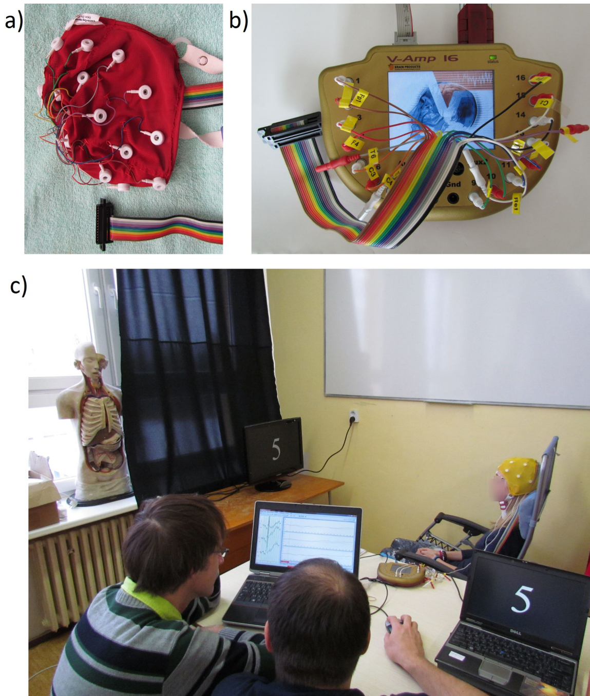
Figure 9.42: a) Medium 10/20 EEG cap. b) The BrainVision V-Amp amplifier. c) Course of the 'Guess the number' experiment. Researchers observe event-related potentials while they are averaged in the BrainVision Recorder. The notebook on the right was used to control the stimulation. The subject sitting in the chair is exposed to visual stimuli. The subject's face has been blurred to protect his/her privacy.
