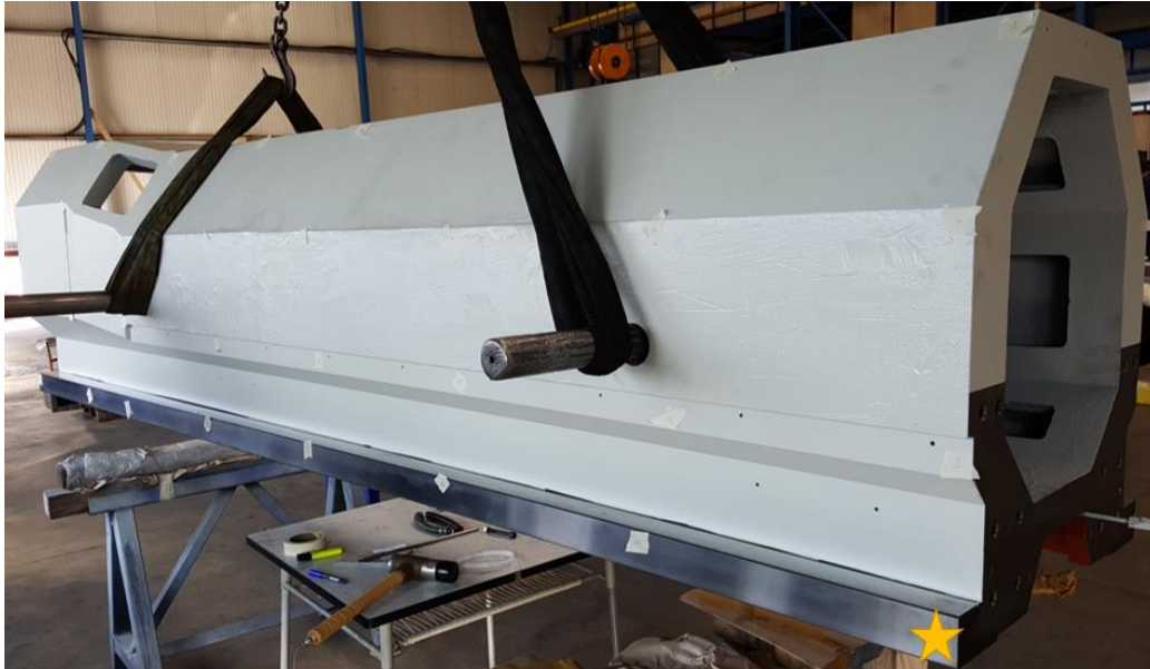
Fig. 12 - The ram hung on ropes (prepared for measurement)
