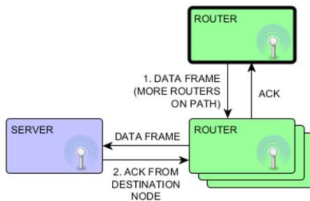
Figure 6 Delivering router to server communication
