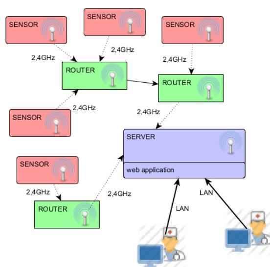
Figure 1 Topology of wireless system
