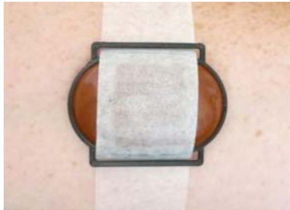
Figure 2 Wireless temperature sensor fastened on skin
