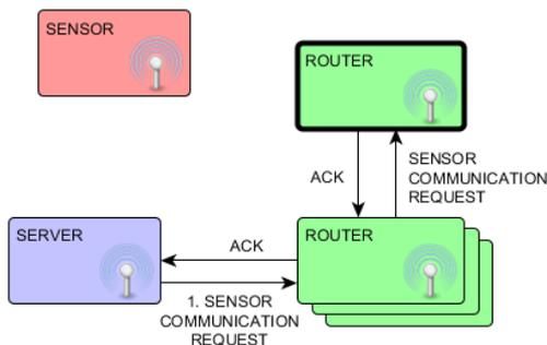
Figure 7 Request for communication with sensor
