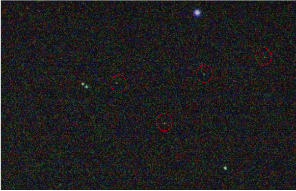
Figure 6. Gamma correction of previous image for better visualization of other recognized stars and residual thermal noise. Red circles show newly recognized stars.
