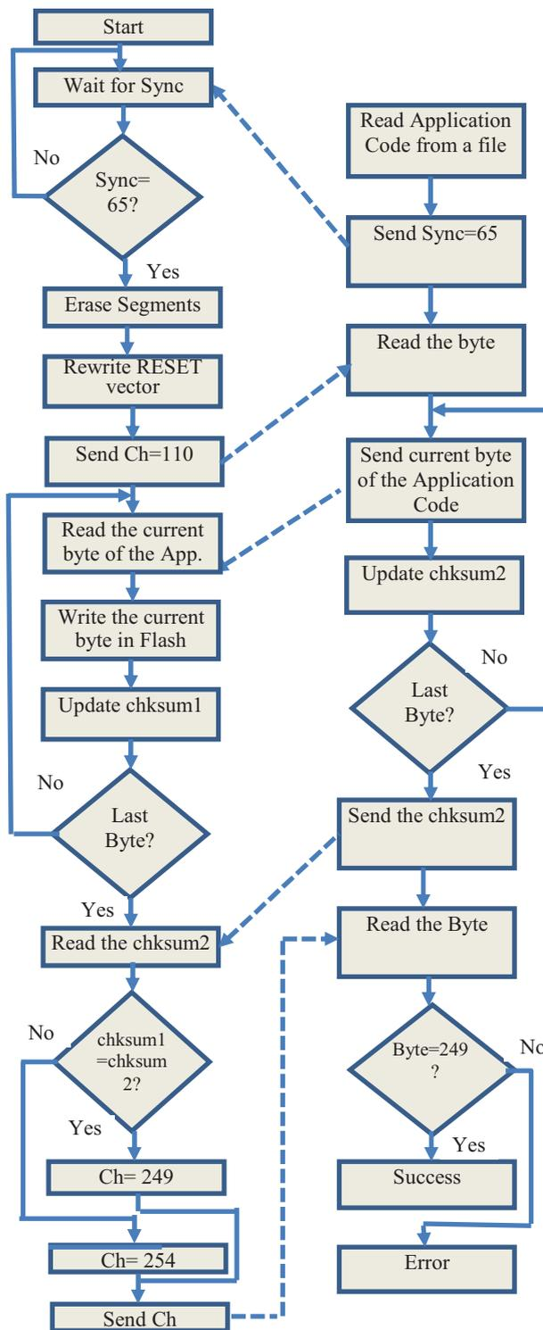
Figure 4. MCU (left) and PC-MATLAB (right) algorithms
