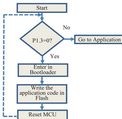
Figure 1. The architecture of the MCU software
