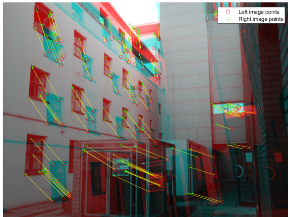
Figure 26: Feature matches after filtering false matches using RANSAC. The matched points are visualised on the right image by drawing a line from the left image point to the right image point.
