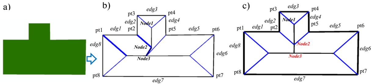
**Figure 3: a) An orthogonal building polygon b) a monotone polygon with an acute angle c) rectified monotone polygons by ‘Line segment’ event**
