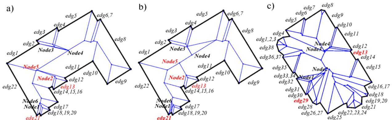
**Figure 5: Monotone polygons with acute angle and self-intersecting monotone polygons.** a) Some monotone polygons have acute angle if a Line segment event does not occur. b) & c) Some monotone polygons are self-intersecting if the set of the nodes are sorted according to the 'node vector projections' onto the original edge vector.
