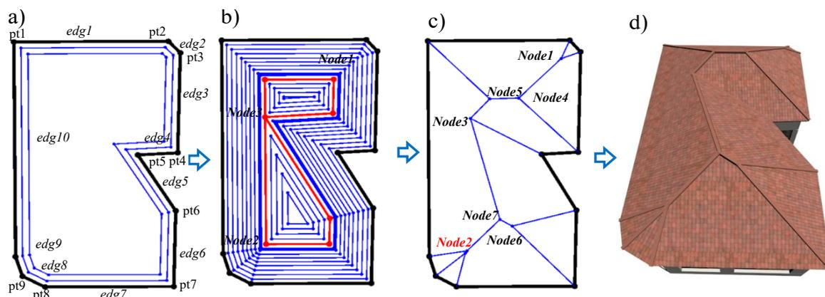
**Figure 2: Shrinking process and a straight skeleton, a roof model generated. a)** Input polygon (bold) start continuous shrinking process in which edges of the polygon move inward, parallel to themselves at a constant speed. **b)** Shrinking polygons (blue) by no event, and red one by a split event. **c)** The straight skeleton (blue) and monotone polygons. **d)** A roof model automatically generated: each roof board is based on an ‘monotone polygon’.
