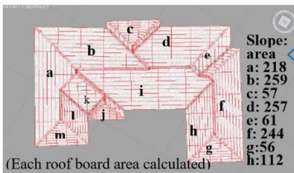
(i) Automatically created roof report for damage evaluation
