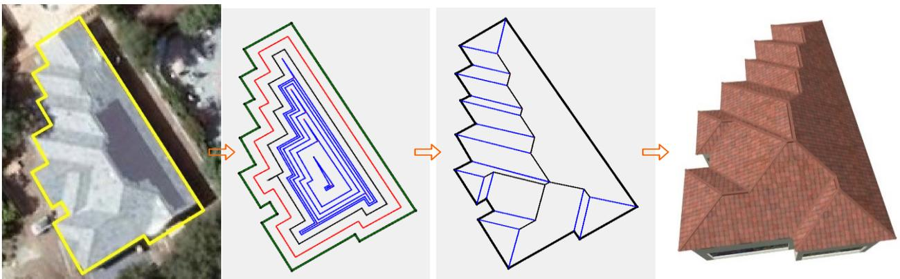
(e) Enlarged building polygons: orthogonal (f) Set of receding polygons by  $d_{shri}$  calculated by equation (1) (g) The straight skeleton formed as the union of the pieces of angular bisectors (h) Automatically generated 3D building model based on monotone polygons
