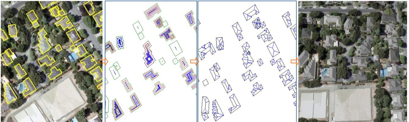
(a) Building polygons on 2D Digital Map: Most of them are orthogonal. (b) Set of receding polygons by  $d_{shri}$  calculated by equation (1) (c) The straight skeleton formed as the union of the pieces of angular bisectors (d) Automatically generated 3D building model based on monotone polygons
