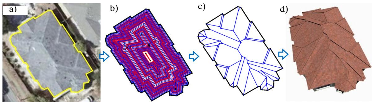
**Figure 6: Complicated shape polygon in shrinking process and a straight skeleton, a roof model generated.**
