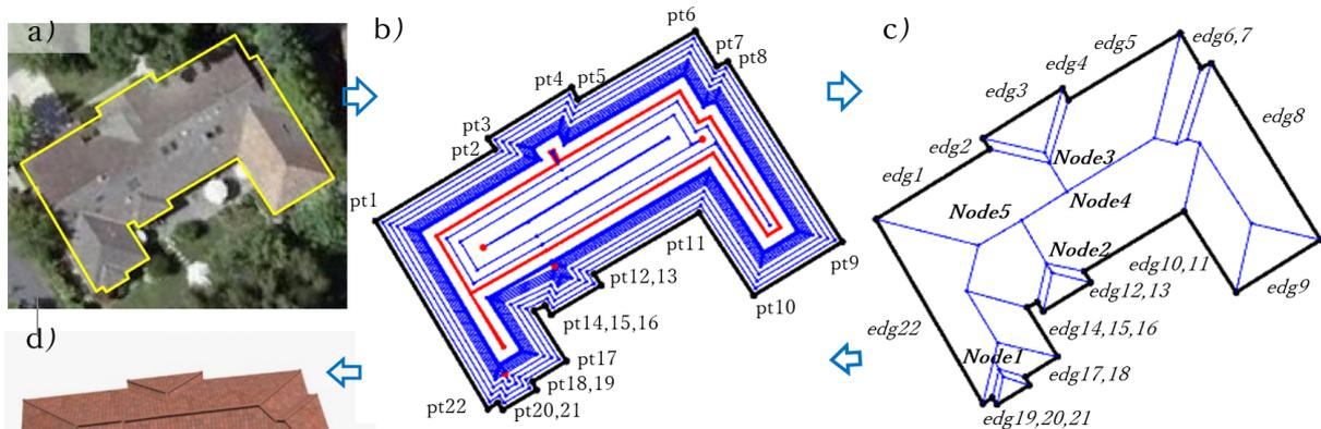
**Figure 4: Orthogonal building polygon in shrinking process and a straight skeleton, a roof model generated.**
