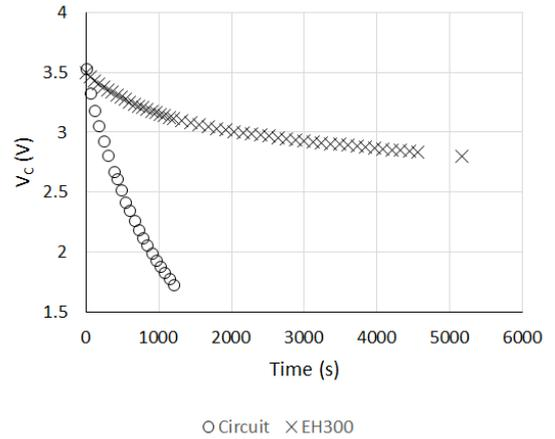
Fig. 3: Measurement of the voltage drop on the storage capacitor during the time caused by the leakage currents
