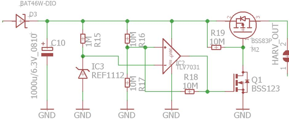
Fig. 2: Schematic of the harvester circuit
