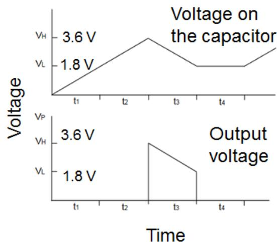
Fig. 1: Operating cycle of the harvester EH300 [2]
