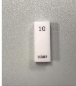
Fig. 3. 10mm ceramic gauge block
