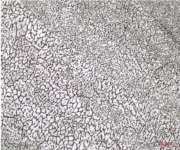
FIGURE 5: ‘85 % Cu, 15 % metal oxides’; ZONE 3; dendritic structure with notable interdendritic spaces consisting of copper; etched; magnification 1000×
