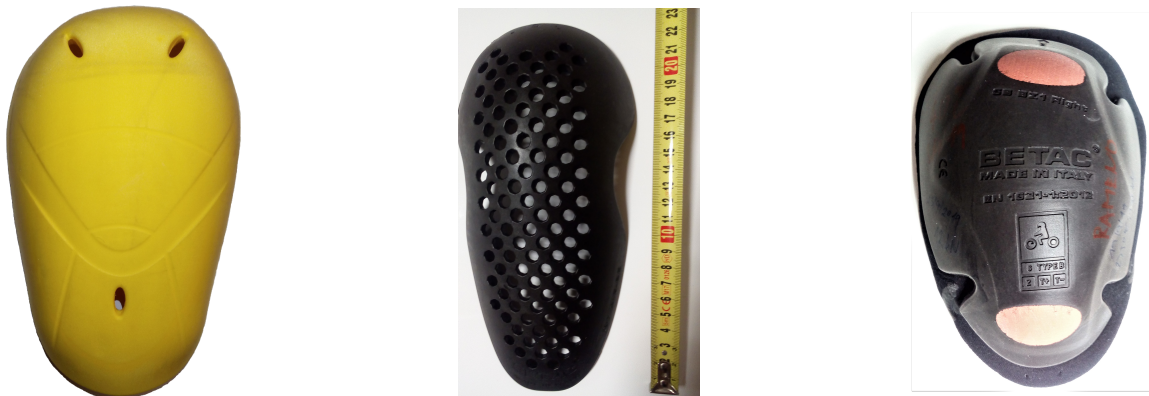
Fig. 1. Joint protectors: (a) SAS-TEC SCL-2, (b) BETAC with perforations, (c) compound BETAC
