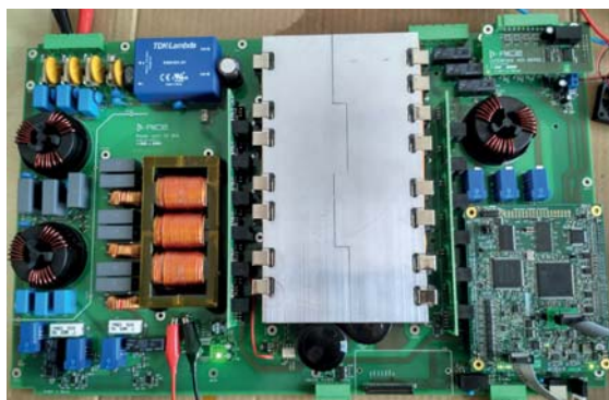
Fig. 7. First revision of converter hardware
