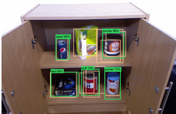
Figure 6: Sample result of object detection: yellow boxes – RPN result, green boxes – detected objects.
